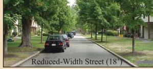
Streets as narrow as 18 feet provide ample two-way driving space for low-volume streets, while forcing traffic to slow down, reducing pedestrian crossing time and leaving more room for open space<sup>1</sup>.
