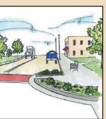
On-street parking provides access to businesses while narrowing the travelled way and calming traffic. Often seen in combination with on-street parking, curb extensions narrow the roadway, shorten pedestrian crossings and improve vehicle sight lines.
