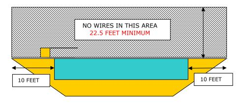
No overhead wiring shall be installed within **22.5 feet (6.9 m)** vertically from the water and all areas extending **10 feet (3.05 m)** horizontally from the inside of the walls of the pool. Wiring above diving structures, observation stands, towers, or platforms shall not be within **14.5 feet (4.40 m)**.
