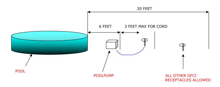
NOTE: IF USING A RECEPTACLE FOR THE POOL PUMP, IT SHOULD CONSIST OF: GROUNDING, WEATHER-PROOF TYPE, and GFCI PROTECTED
